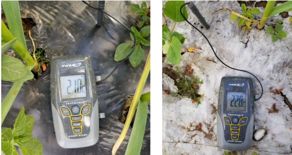
Figure 3: Measuring soil temperature under black plastic and paper mulches. Photo credit M. Carr; June 4, 2018.
